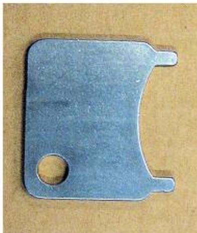
This tool is used for removal and refitting of spray nozzles only
