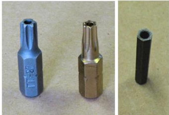
T27 (left) is used for removal of the new-style soap lid (from 2012 onwards)
